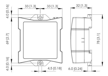
Figure 5: Dimensions in mm [inch]
